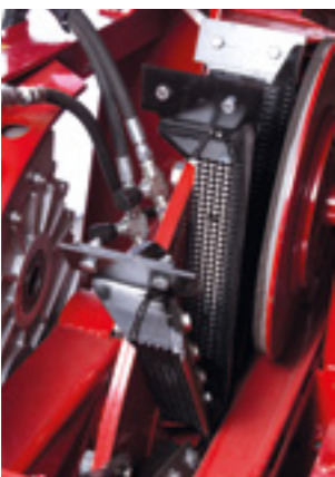
Blade holder with cracker.
